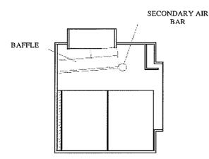
1. Ensure the ceramic baffle blanket is fitting flat on the top Face of the Baffle.
